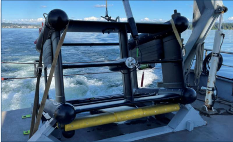
III eBOSS is an advanced sub-bottom sonar system capable of penetrating the seabed to accurately detect, locate, classify, and identify buried and partially proud objects. This low-frequency acoustic imaging system provides data in real-time for general survey purposes such as cable & pipeline depth-of-burial tracking and route surveys. Data can also be post-processed utilizing synthetic aperture sonar (SAS) processing and beamforming to render 3-dimensional images of buried objects.
